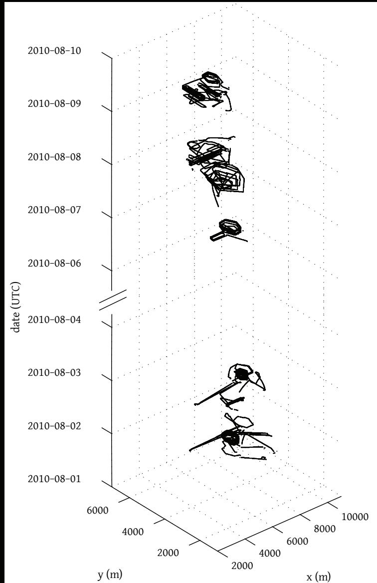
Position of single AUV doing many different missions over 60+ hours
