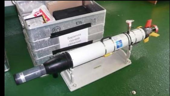
Hammerhead (Iver AUV)
