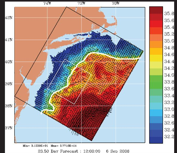
First, develop a simulation using one AUV in a dynamic ocean model environment to detect & track a 2D front boundary...
