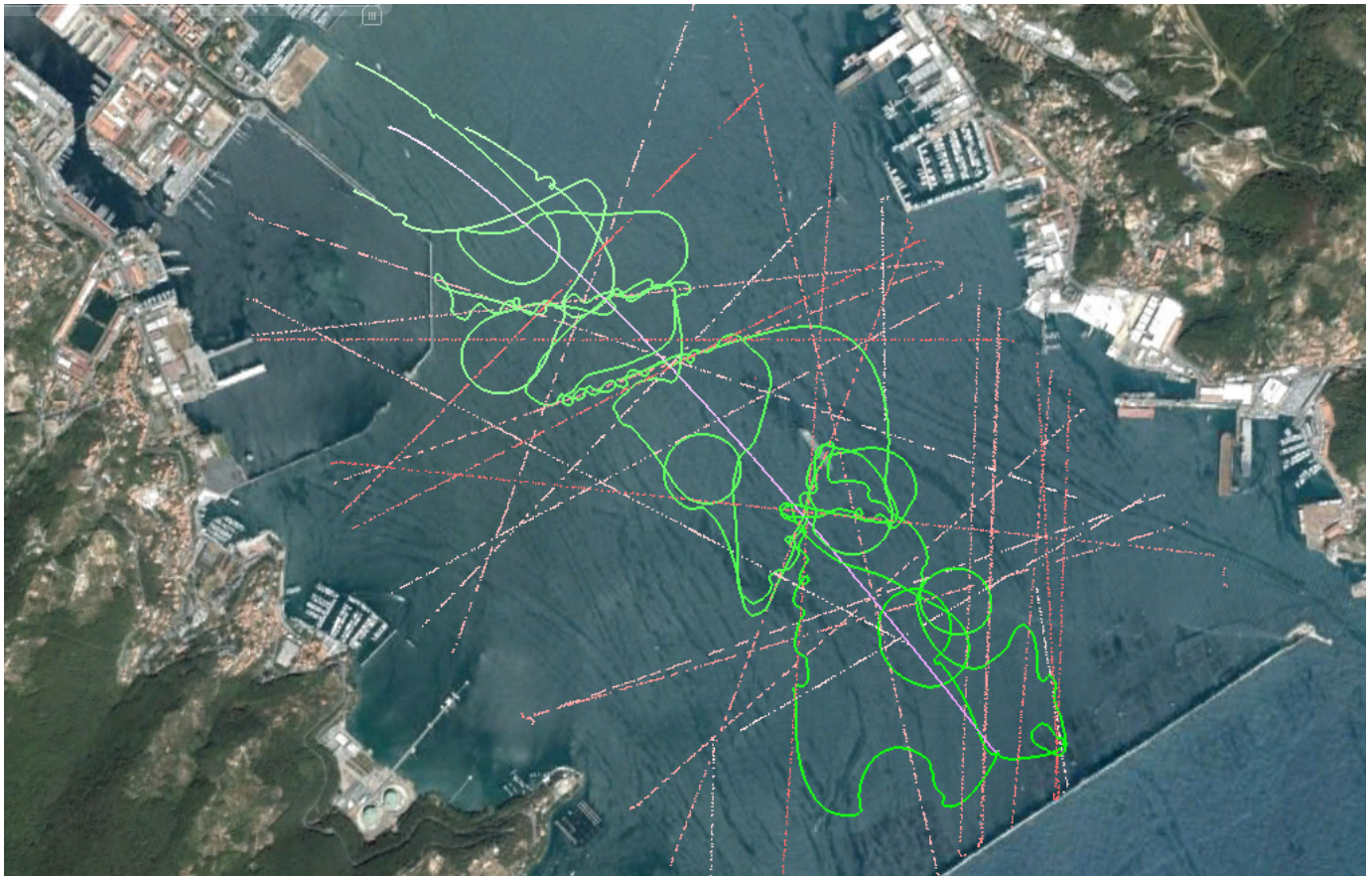
Fig. 4: Simulation of cluster defense of three USVs (green) protecting one ship (purple) from many potential targets (red). The ship has transited from the bottom right (near the seawall) to the upper left. The colors fade from dark (start of mission) to light (end of mission). See Fig. 5 for a snapshot view of this mission. Throughout the mission, the USVs have actively investigated many potential targets. The parameters used in this simulation are given in Table I.
