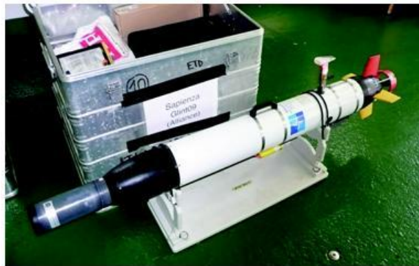
Figure 16. The NUWC 'Hammerhead' Iver AUV used during Champlain '09. This AUV carries a complete environmental package in its nose and communicates with the ship via RF (on the surface) and acoustics (underwater). It also carries a GPS and Doppler Velocity Logger (DVL) for positioning. Used with permission from (Petillo, Balasuriya, & Schmidt, 2010).
