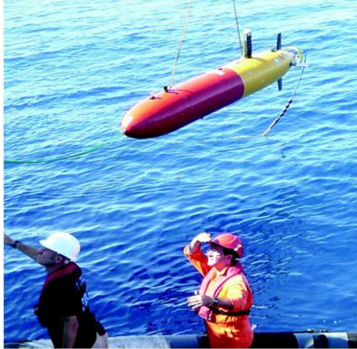
Figure 13. The NURC OEX AUV during GLINT '09. This AUV uses acoustics to communicate with the ship while underwater and gets position updates via GPS when surfacing. Used with permission from (Petillo, Balasuriya, & Schmidt, 2010).
