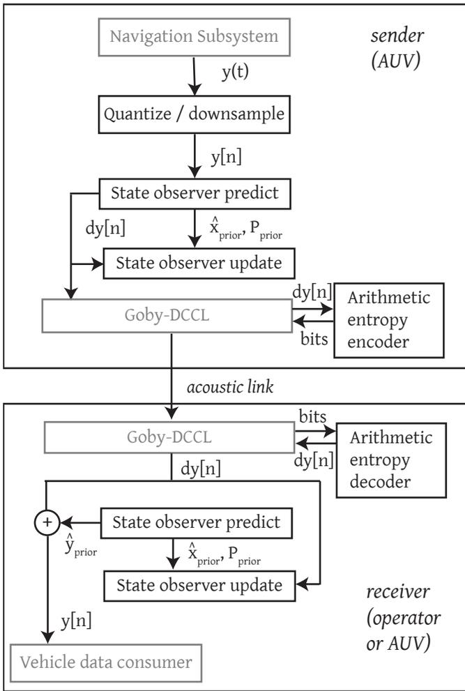
Fig. 2: Data flow for the delta transmission part of the encoding system presented in this paper. Gray blocks are subsystems not presented in this paper. Section III presents the state observers, and section IV elaborates on the arithmetic entropy encoder. Goby-DCCL is discussed in [16].
