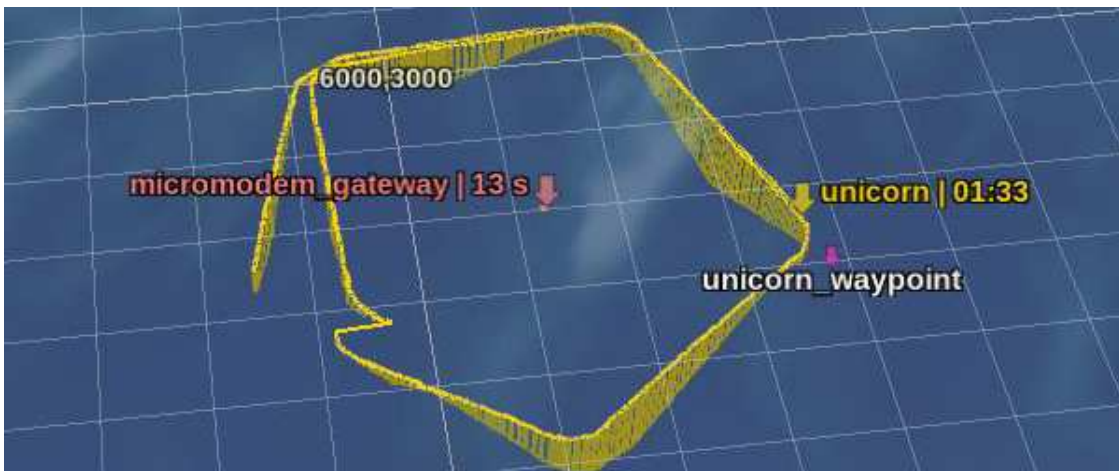
(b) A snapshot of the runtime visualization of the AUV “Unicorn” performing a sinusoidal depth excursion while performing a pentagon shape. While full updates are delayed, the LAMSS_STATUS_FILLIN and LAMSS_CTD messages give a detailed history of the vehicle’s track when the communication environment permits.
